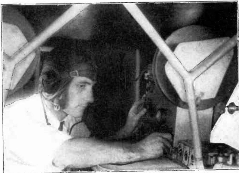
Lt. Malcolm P. Hanson, chief radio engineer of the Byrd Antarctic expedition, in the cabin of the "Stars and Stripes." Notice the two aerial wire reels at the right and left.
