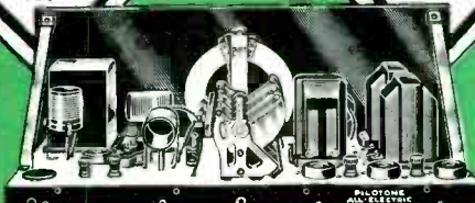
ONE OF THE NEWLY DEVELOPED PILOT KITS. AN A-C JOB WITH PUSH-PULL AMPLIFICATION AND BUILT-IN "A" POWER
