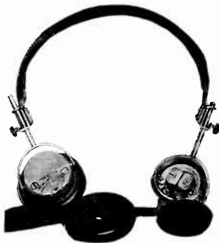
A pair of standard earphones. The phone on the right has been opened to show the screw cap (center) and the diaphragm (right).
